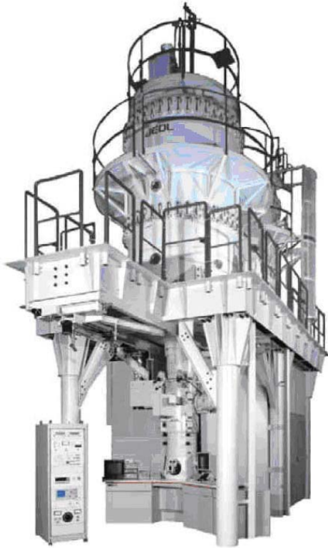
Fig. 1. High voltage electron microscopy set up in KBSI (Korea Basic Science Institute, Daejeon, Korea) (JEM-ARM 1300S, JEOL; Maximum accelerator voltage: 1.3 MV).
