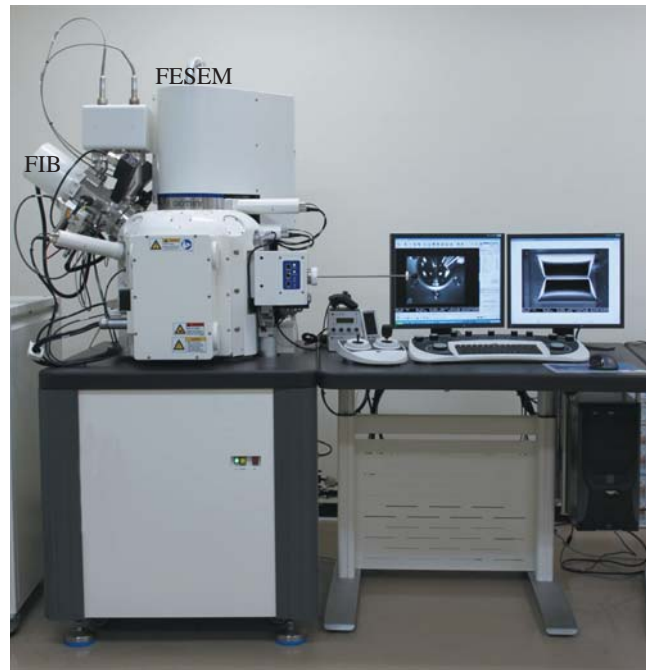
Fig. 1. Modern FIB-FESEM. An FESEM column is located in the middle, and an FIB column is installed in the left side of the system.
